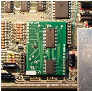
The circle printed in the top left hand corner of the face of the upper RAM module must be placed directly over contact 1 of the socket in position IC22. The module's lower rightmost pin must be inserted in contact 9 of the socket in position IC15. The leftmost column of contacts of the socket in position IC18 and the rightmost column of contacts of the socket in position IC19 are not covered by the upper RAM module.
