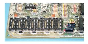
The connecting pins should be perfectly perpendicular to the lower surface of the module's circuit board. Use thin-nosed pliers to gently straighten any that have become bent during transportation or storage.
